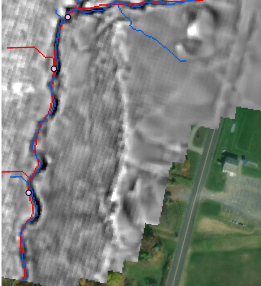
Figure 1. Example of the E_{dif} layer on a black (deposition) to white (erosion) color scale, along with the concentrated flow path from 2006 (in blue) and 2017 (in red). Note that in nearly all bends of the channel, the 2017 channel is straighter than the 2006 one. E_{dif} on the outside of the bends is black, indicating deposition, which pushes the stream channel towards the inside of the bend, thus straightening it. The pink dots are carpet locations. Scale of the map can be inferred from the two-lane road and parking lot visible in the aerial photo visible on the right side of the figure.
