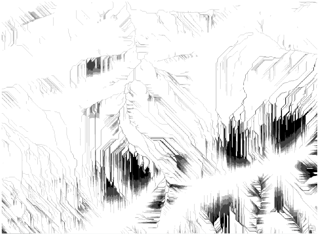
Figure 3. Map of T_c , ranging from low sediment transport potential (clear) to high (dark). The land area is the same as that shown in Figure 2. Darkest areas are near the base of steep hillsides
