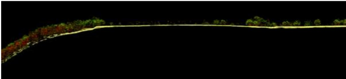
Figure 4. Sample LAS Profile depicting class 12 (green) as well as the selected returns for class 1 (red) that represent vegetation. Building rooftops are omitted.
