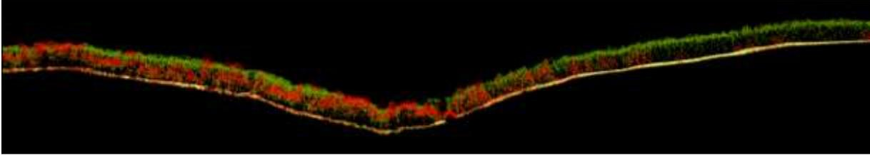
Figure 2. Sample LAS profile for a forested area. Green points are class 12 (overlap/reserved), while red ones are class 1 (unassigned)
