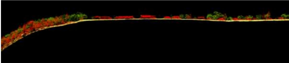
Figure 3. Sample LAS profile depicting class 12 (green) as well as mixed class 1 (red). Building rooftops as well as some mid to high vegetation covers are both shown in red.
