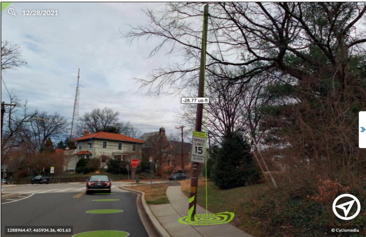
Step 6: The height of the cable from its lowest point to the sidewalk is **28.77** feet. According to the new DDOT regulations, this cable does not meet the minimum height requirement, and will have to be removed and replaced.
