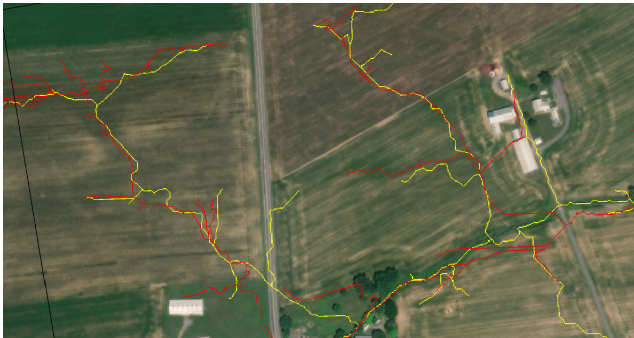
Figure 3. Yellow (red) lines represent 2006 (2017) flow paths. Distance between the start of corresponding paths is one measure of soil displacement considered here.
